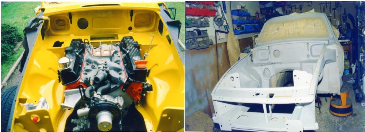
The body shell was completely dismantled all items were removed apart from the dash and steering wheel. Rust repairs were completed where necessary, the whole body was prepared and undercoated then painted with cellulose lacquer. Underseal was applied front to back.
