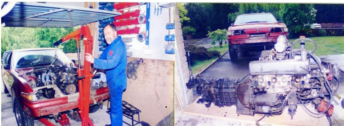
While living in Cardiff, John removed the engine, cleaned stripped and re-conditioned it, altering carburettor, oil filter and sump plug positions to suit the BGT engine bay. With the help of the MG Centre workshop Cardiff, parts from Rimmer Brothers and other suppliers and repair shops, he purchased new and reconditioned parts and proceeded to work from the front to the back of the car converting all components to factory BGT V8/SD1 specifications, including:
