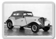
**Produced** 1949-53; **Value** £9500-14,000 New two-seater sports design, with independent front suspension and rackand-pinion steering, as on Y-type. 1250cc four-cylinder, ohv engine (as in TC), 54.4bhp at 5200rpm. Bolt-on-disc wheels (pierced on later cars).TD MkII available (1950 on) with increased power (57bhp at 5500rpm) and optional centre-lock wire wheels. Approximately 30,000 built.
