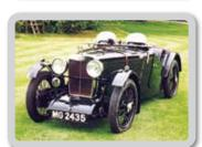
**Produced** 1932-34; **Value** £10,000-16,000 Further development of M-type. 847cc, four cylinder, ohc. 36bhp at 5500rpm (II and J2), 746cc supercharged (J3 and J4). J1, four-seater; J2, two-seater; J3, supercharged; J4, supercharged racing model (72.3bhp at 6000rpm). Four-speed gearbox. Centrelock wire wheels. Some had swept wings instead of cycle-type. Approximate numbers built: | 1/|2, 5500; |3/|4, 30.
